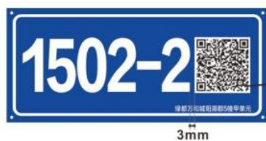
整体尺寸169x74mm 内框尺寸157x62mm 数字编号字号113pt 字间距-15% 总长度108mm
